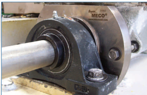
MECO Seal on Auger Packer
