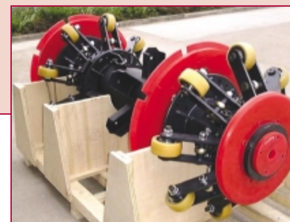
Fig 4. 36 inch fixed diameter pipe line cleaning/gauging system
