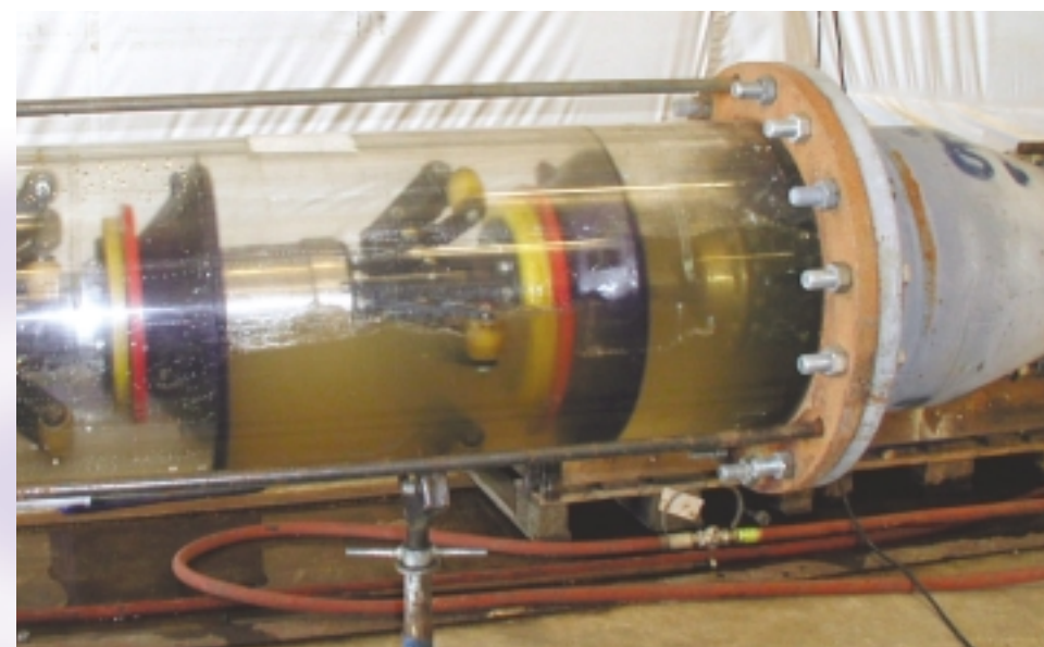
Fig.2 Norne Heidrun Optopig® test vehicle entering the 16inch spool piece. Note the even contact of the suspension wheels and the front drive disc holding back the water, used to drive the pig in this simulation.
