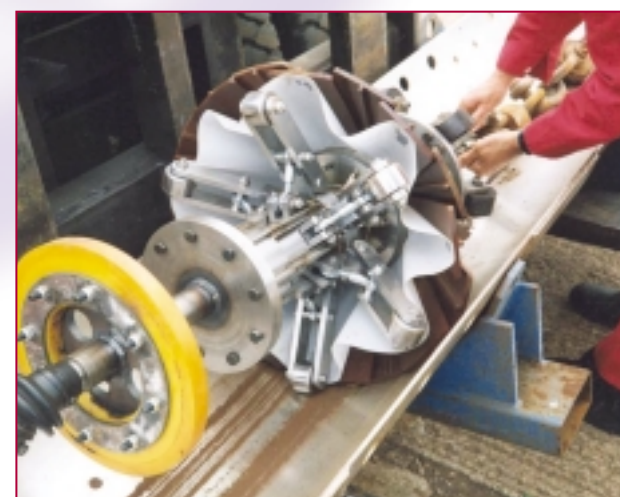
Fig.3 Varipig being used as a tow module on the front of a MFL tool.
