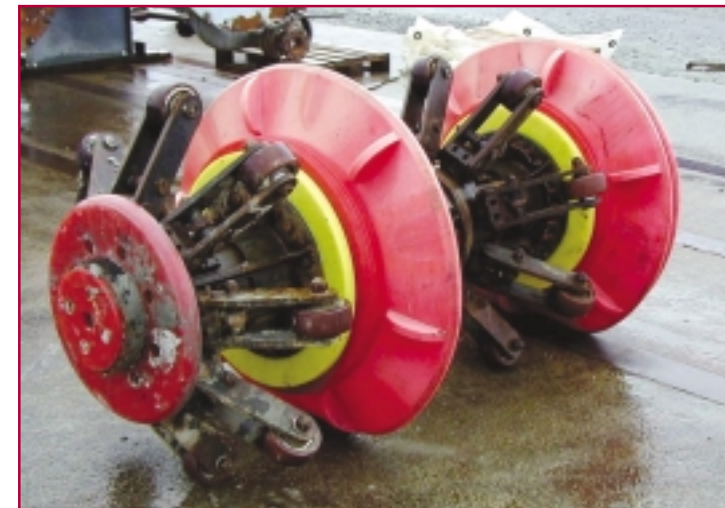
Fig.1 One of the six Åsgard pigs following its 700+km dewatering run
